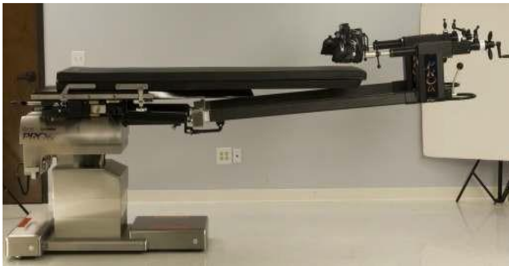
Figure 42. ProFx® Table Shown with REF 6850-6000 Auxiliary Imaging Top : The Auxiliary Imaging Top is shown attached in Position 2, fully adjusted towards the foot end of the table with both leg spars attached to the table. It is important to note that the Auxiliary Imaging Top can be installed onto the ProFx® with one or both leg spars attached to the table to facilitate traction.
