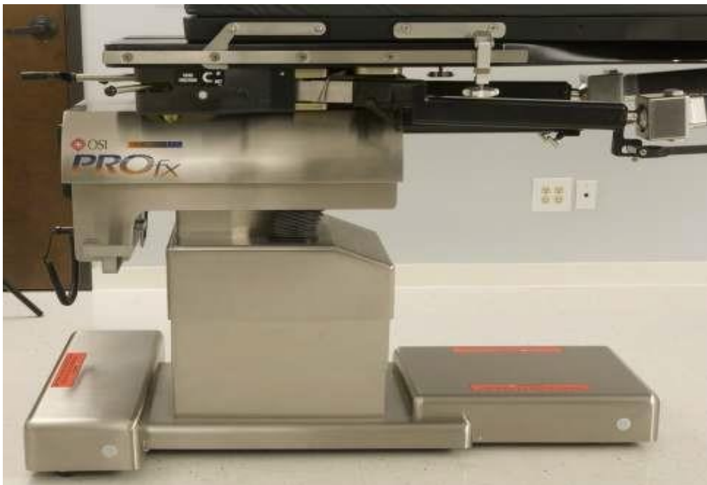
Figure 40. ProFx® Table Shown with REF 6850-6000 Auxiliary Imaging Top: The Auxiliary Imaging Top is shown attached in Position 2, fully adjusted towards the foot end of the table with both leg spars attached. It is important to note that the Auxiliary Imaging Top can be attached to the ProFx® Table in two positions: Position 1 for normal imaging range, and Position 2 for extended imaging range when needed.
